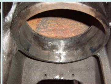
The third direction of the repair that was performed simultaneously to the restoration of the other two parts of the generator, damaged during an accident, was the cylinder liner of forth motion, particularly in the area below the packing surfaces of the cooling space.
