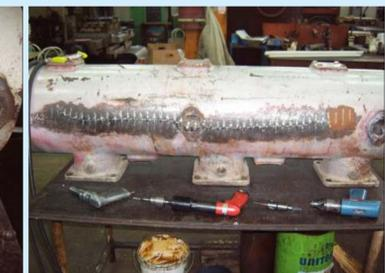
The crack is locked, then final packing of material is performed, cutting out and grinding of the redundant metal. (fig.4)
