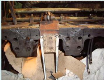
The damaged part to which new material was added as to enable restoration of casing wall. The new detail was fabricated of cast iron and was embedded in the broken part of the casing, using the METALOCK method. (fig.7)
