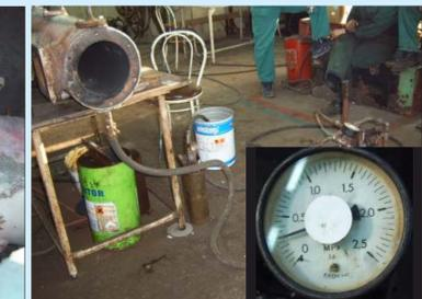
Moment from the hydraulic test of the cooling space in the collector casing. The indicator of the manometer shows 0,3MPa. (fig.6)
