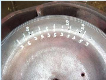
Restoration of cylinder block wall. (fig.5)
