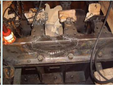
Repaired casing wall through the METALOCK method. Casing surfaces that is in contact with the surface of the cylinder block is grinded to roughness and flatness, similar to that of the other part. (fig.13)
