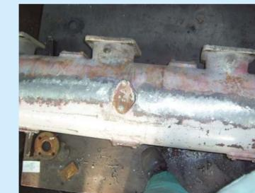
Surface of the collector's casing after final completion of repair (fig.5)
