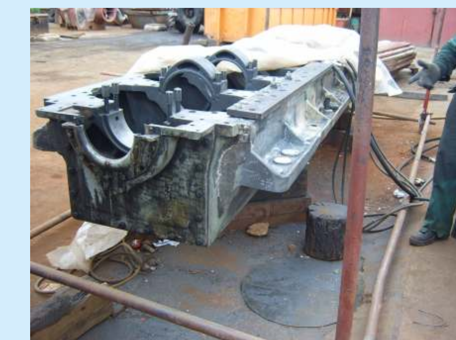
Aligned new part. Tightened and ready for embedment through the Metallock method of repair (fig.10, 11 and 12)
