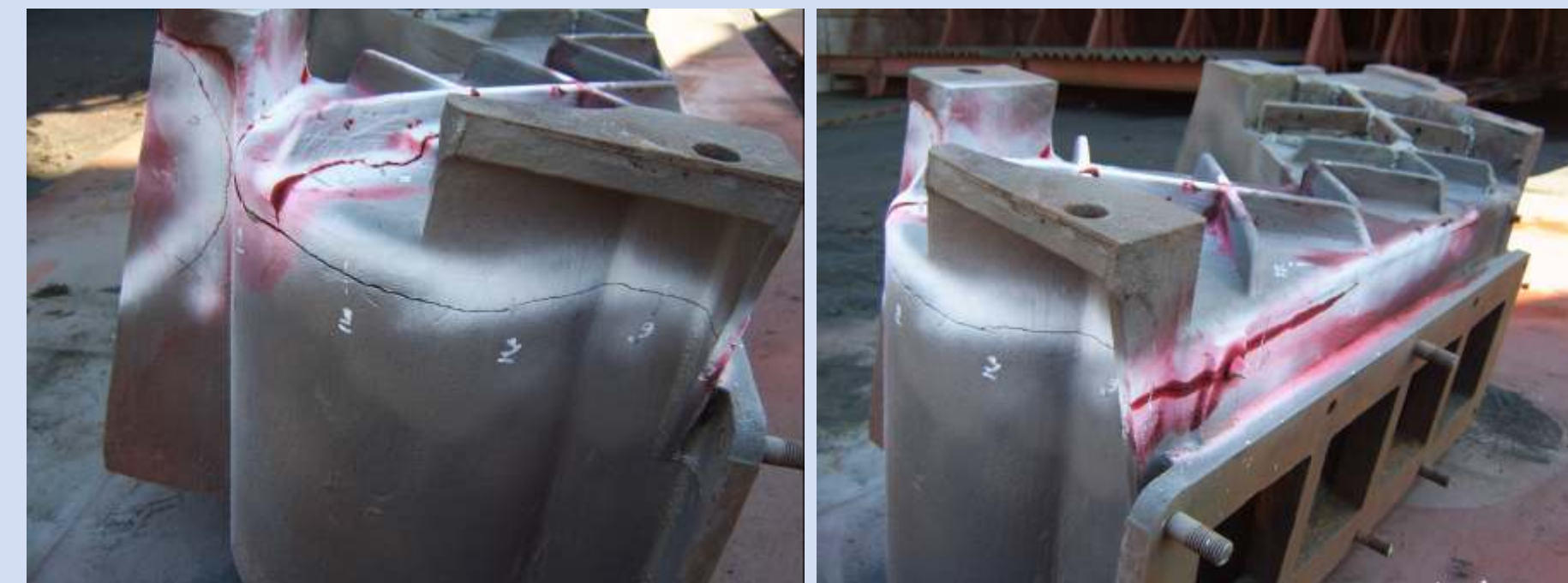
Condition of pump casing at delivery for repair (fig. 1 and 2)
