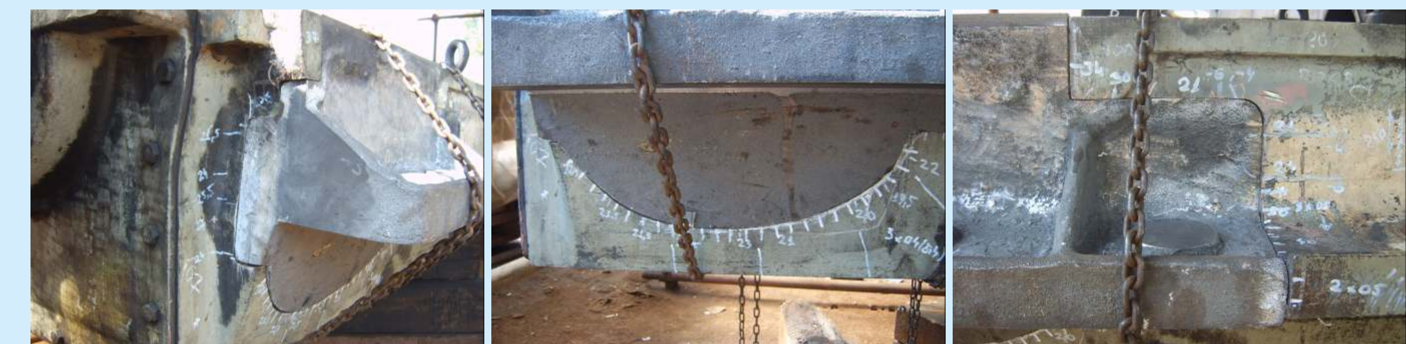
Aligned new part. Tightened and ready for embedment through the Metallock method of repair (fig.10, 11 and 12)
