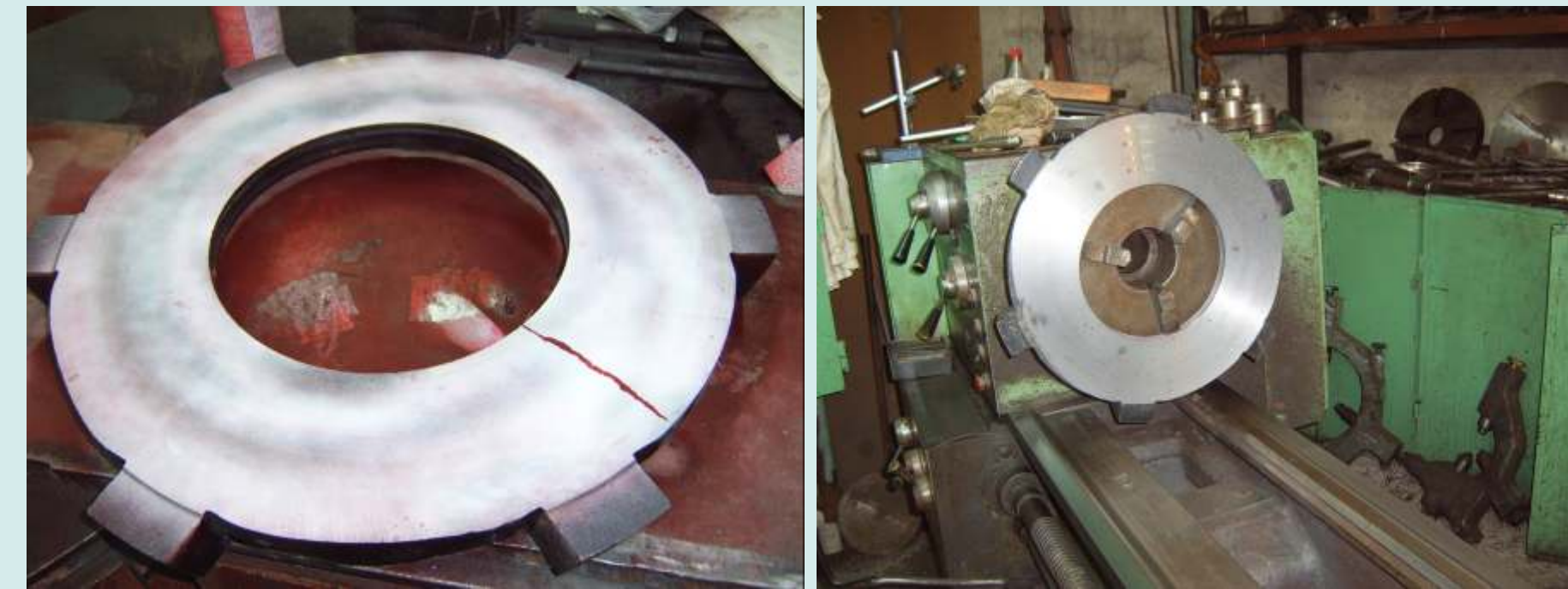
Condition of the disk at delivery for repair (fig.1)
