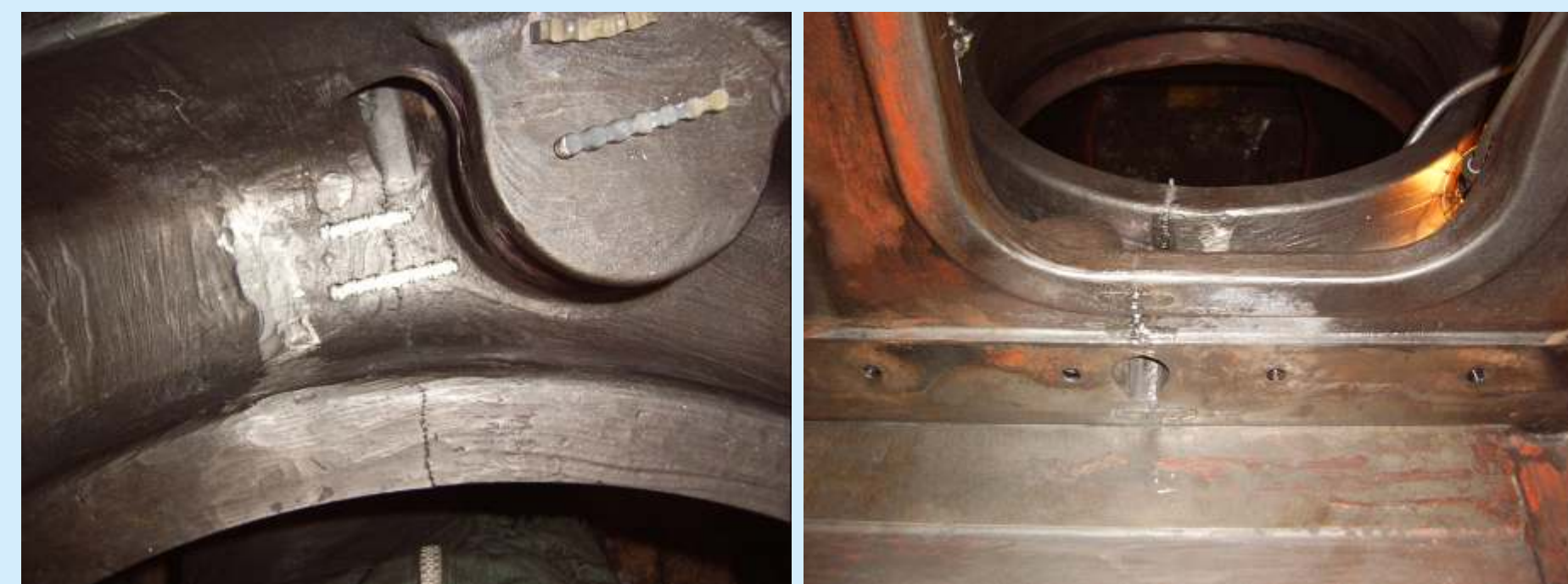
Moments from the Metallock repair on the cylinder block body fig.3 and 4)
